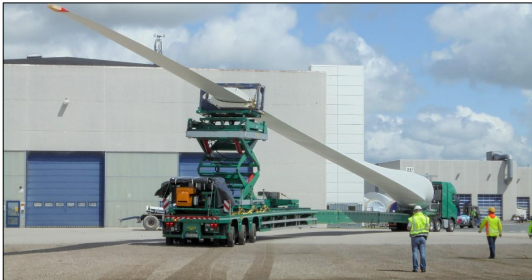
Figure 21. Broshuis 4-Axle Quatro with Lifting and Sliding System
